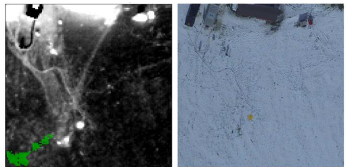
Figure 6. Left: Methane detection over snow covered region. Detected methane plume is shown in green. Right: Corresponding visible imagery from the 12 mega pixels camera aboard the Hyper-Cam Airborne Mini.
