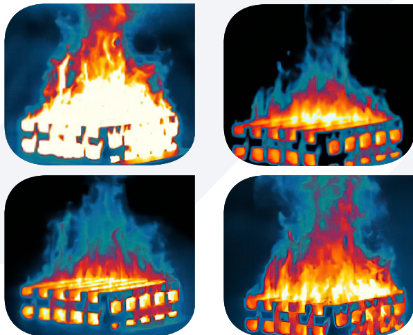
Multispectral image of burning wood crib
