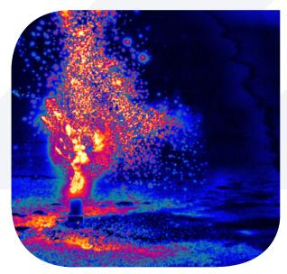
900 degree in-scene dynamic range in a single image allows for efficient measurement of hot targets and cold backgrounds in the same scene
